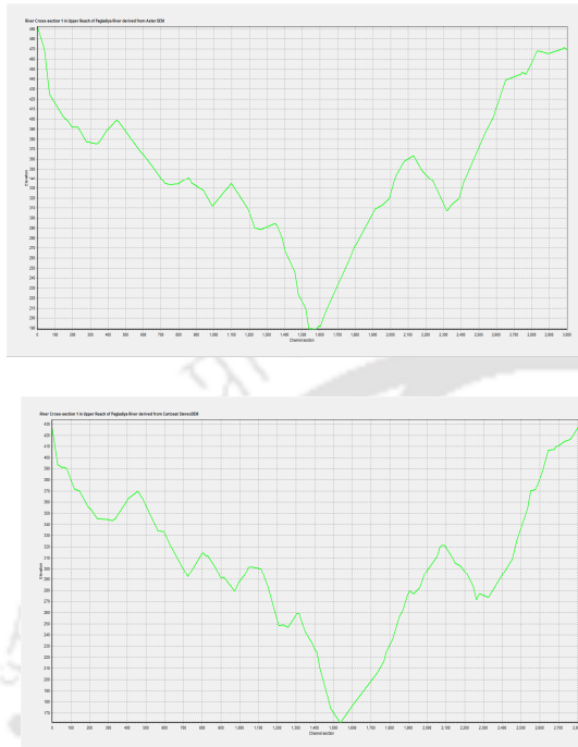
Fig.6.12: A cross section in Pagladia upper reach by ASTER (left) and CARTOSAT-I (right)
