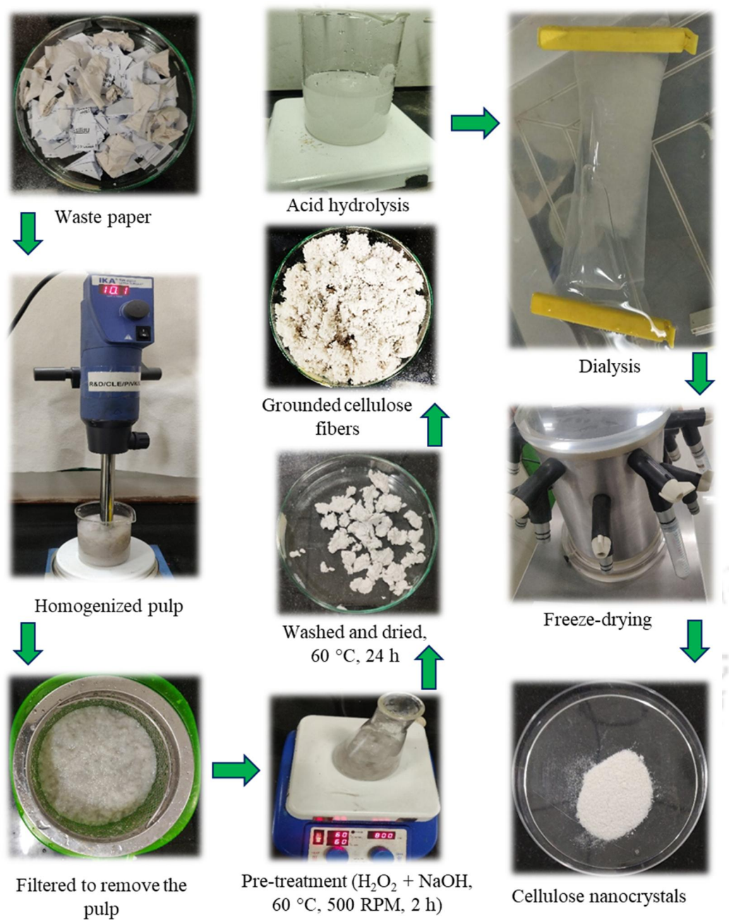
Figure 2.1: Flow chart for pre-treatment of waste paper and preparation of CNCs
