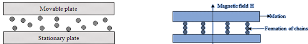
Fig. 1.4: Magnetorheological fluid dampers working principle.
