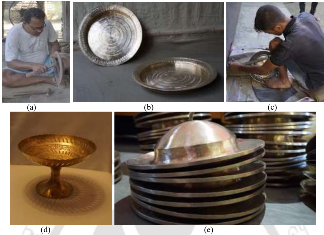
Fig.45 Bell metal producers in traditional producing village (a) Bell metal artist (b) big plates made up of bell metal (c) artist giving final touch to the product (d) a finished product with minute engraving and (e) final products of bell metal
