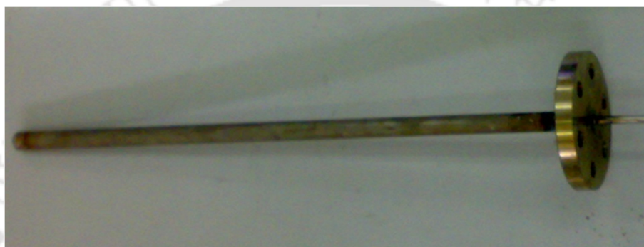
Fig. 4.4 Photograph of SS filter brazed to inner flange.
