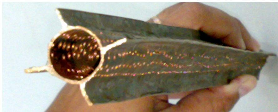
Fig. 4.3 Photograph of copper fin matrix.
