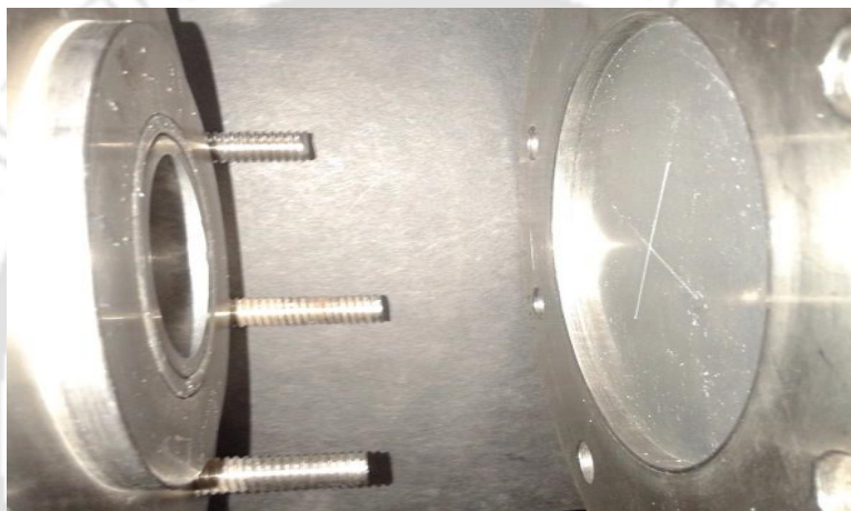
Figure 6.3: Photograph of diaphragm between the driver and driven sections of shock tunnel.
