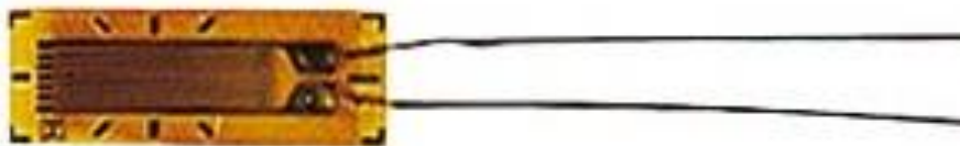
Figure 3.2: Photograph of the semiconductor strain gauge with two leads for connections.
