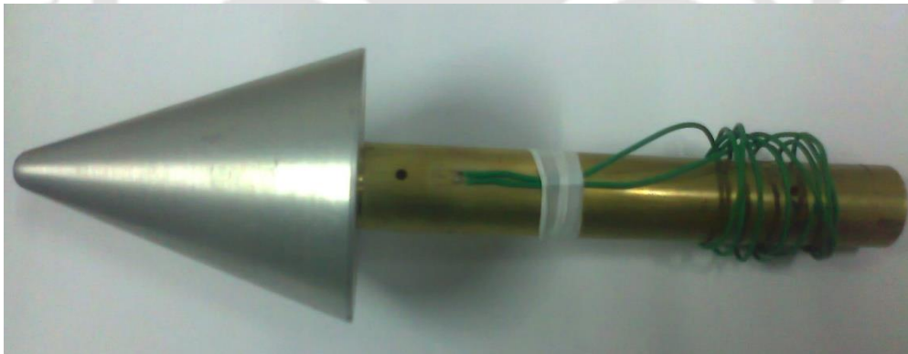
Figure 3.1: Photograph of the strain gage conical model with brass stress bar.
