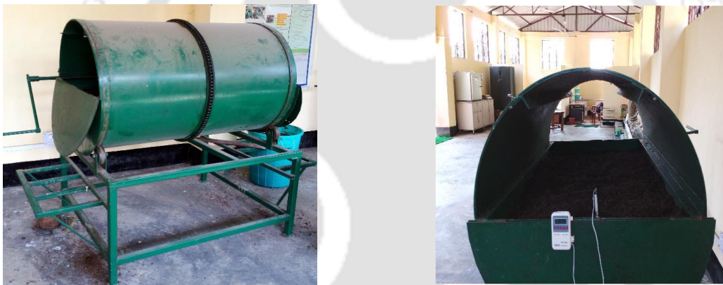
Fig. 4.4. Rotary Drum Composter
