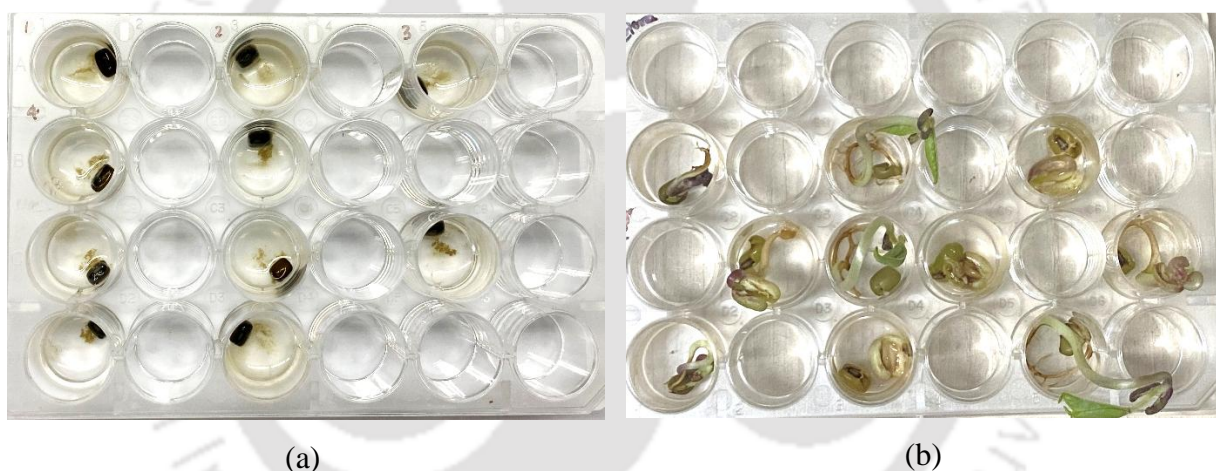
Figure 4.12. Toxicity assay of WW (a) before treatment and (b) after treatment (at the optimized condition: \text{Fe}_3\text{O}_4@\text{AC}@\text{CH} beads dose = 1 g/L, pH = 5.12, \text{H}_2\text{O}_2 loading = 0.75 M)
