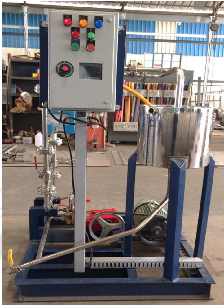
Figure A5.1. Photograph of the hydrodynamic cavitation reactor used in this study
