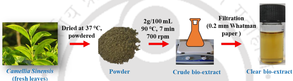
Figure 2.1: Schematic representation of preparation of C. sinensis leaf extract.
