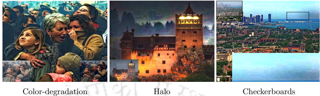
Figure 1.8: A graphical demonstration of the color degradation, halo and checkerboard artifacts in the de-hazed results of existing works.
