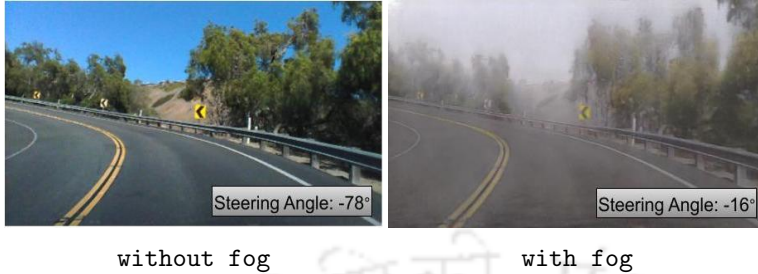
Figure 1.1: Steering angle prediction in the absence/presence of fog by an autonomous vehicle navigation system [1] for the same scene [2].
