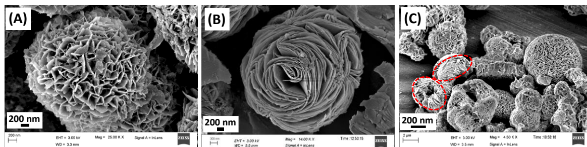
Figure 6: Field emission scanning electron microscopy images of (A) \text{ZnIn}_2\text{S}_4 , (B) \text{VS}_2 and (C) \text{ZnIn}_2\text{S}_4\text{-VS}_2 . Anticipated \text{VS}_2 in \text{ZnIn}_2\text{S}_4\text{-VS}_2 is encircled in red dotted circles in (C).
