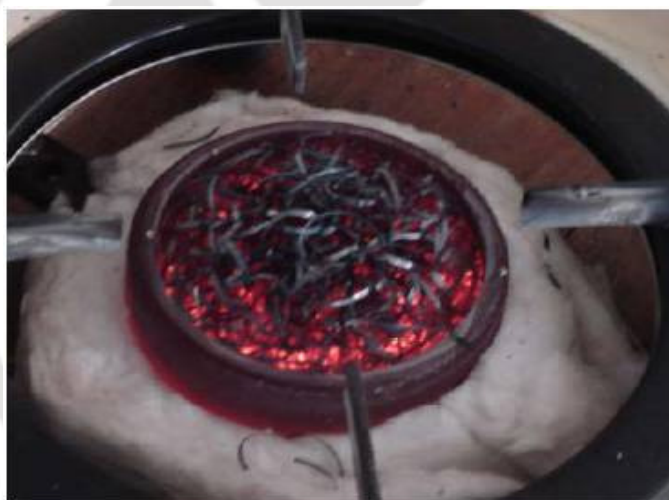
Fig. 3.7 Combustion in porous medium metal chips
