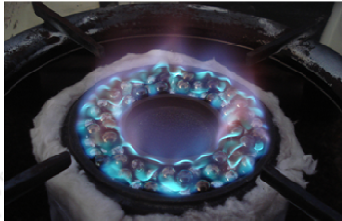
Fig. 3.6 Combustion in the porous medium of metal balls
