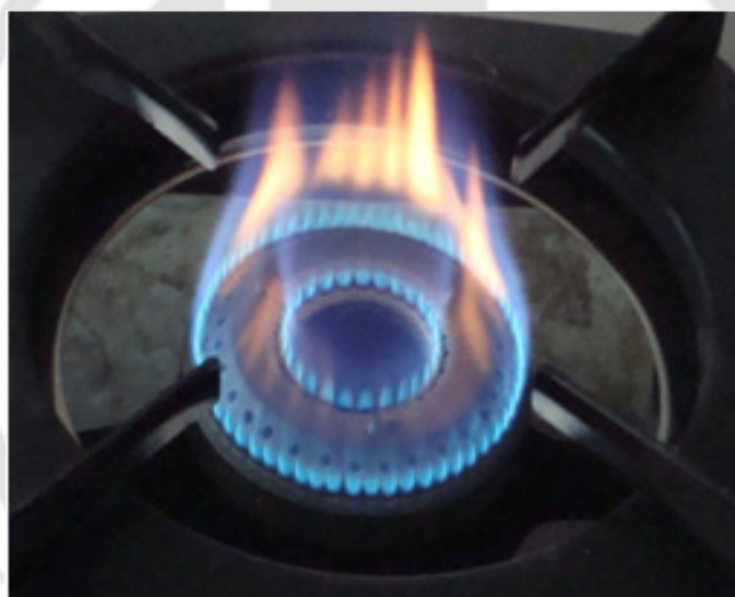
Fig. 2.2 Photograph of the free flame in Conventional Domestic Cooking Stove Burner
