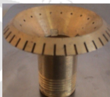
d. Sun-flame Burner
