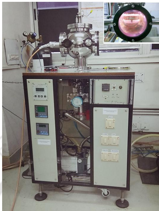
Figure 2.4: rf-PECVD system in our lab (inset image: rf-PECVD chamber during deposition).
