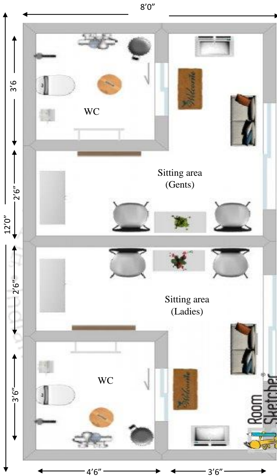
Figure.56. Overview of a final proposed Schematic Diagram (2D concept) of Mobile Utility Van considering both men and women police personnel with an interior plan. (Diagrammatic representation, aspect ratio not locked and not to scale)
