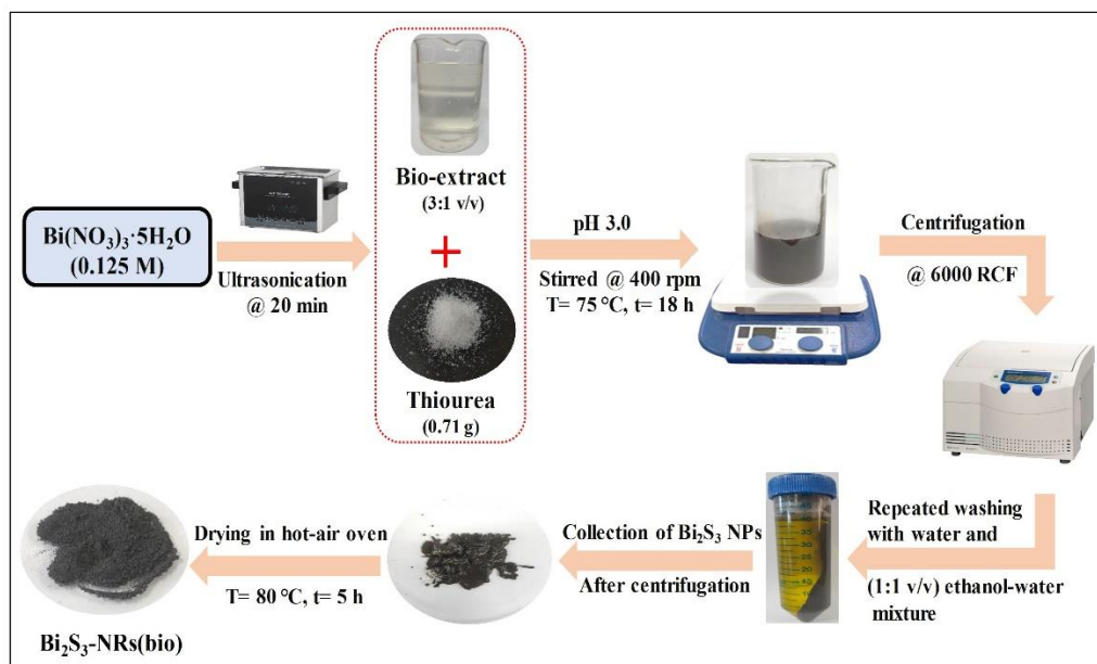
Figure 2.5. Steps involved in synthesizing \text{Bi}_2\text{S}_3\text{NRs(bio)} using Secchium edule fruit extract.
