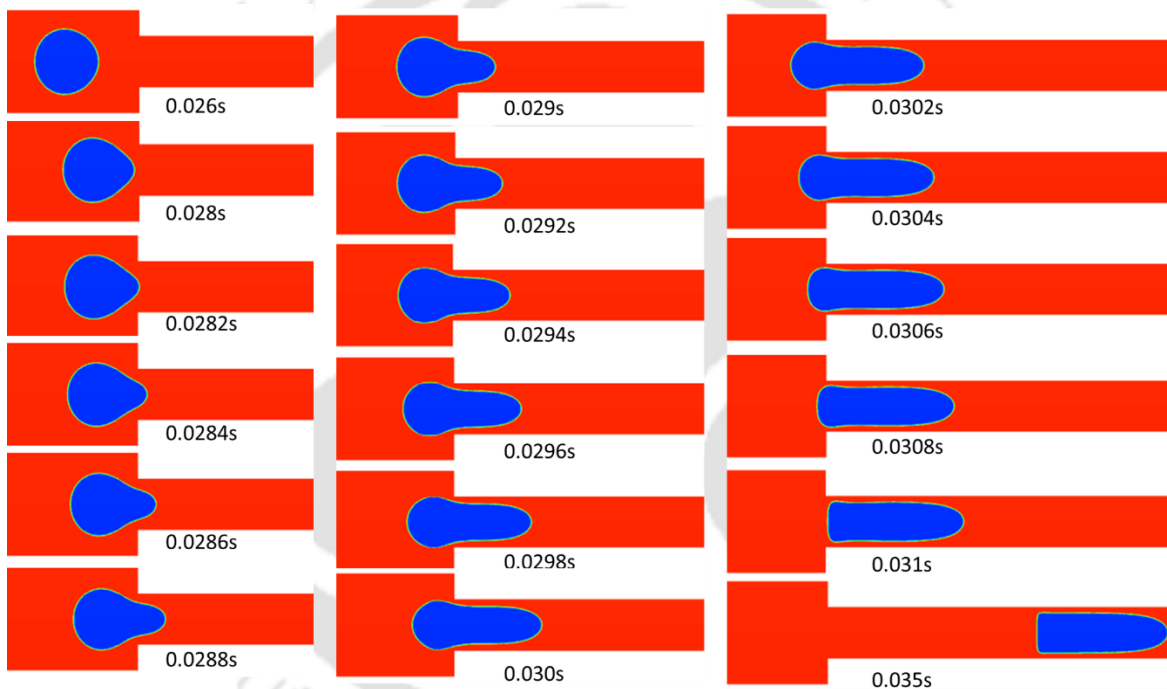
Figure 7.12: Evolution of the bubble shape in a channel of 2 mm diameter having sudden contraction to a channel of 1 mm diameter for a mixture velocity of 0.6 \text{ m s}^{-1} in the 1 mm diameter channel.
