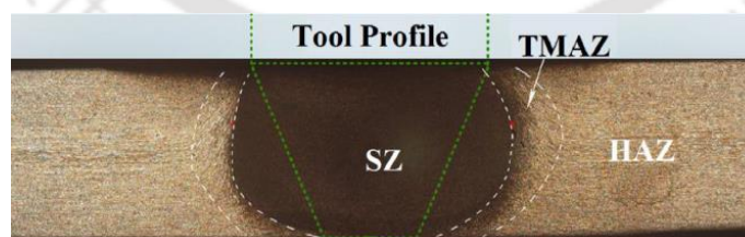
Figure 2.4 Optical macrographs of SSFSWed Al 7075-T651 (With permission from Li et al., 2015. Copyright Elsevier)
