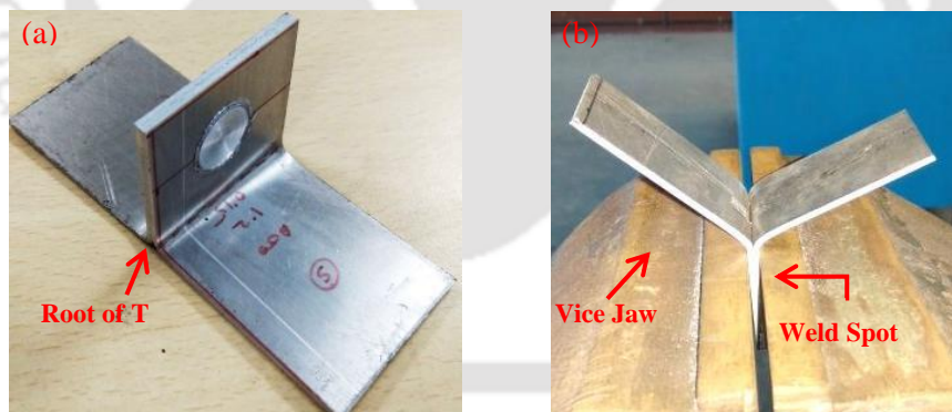
Figure 4.2 Sample preparation: (a) T-shaped sample prepared for T-peel test (b) sample preparation for T-peel test
