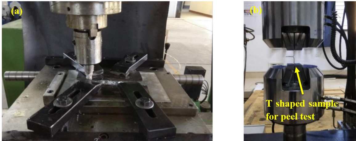
Figure 3.1 Experimental details: (a) FSW machine with integrated force and torque sensors, (b) peel test samples tested in UTM at room temperature
