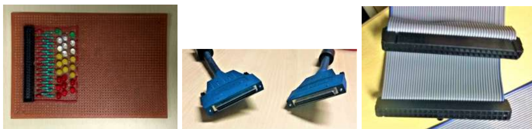
Figure A.1: Image of the LED Board, 68-pin female-female connector, and 50-pin ribbon connector (from left to right).
