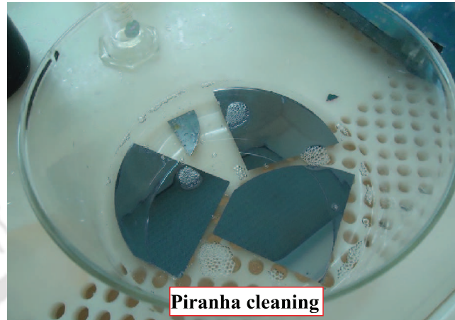
Figure 4.3: The samples are dipped in piranha solution for cleaning.
