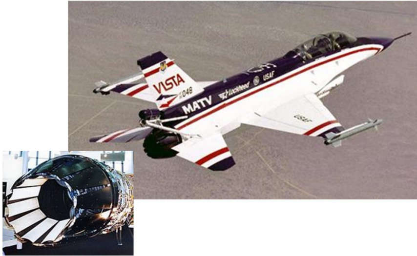
Figure 1.2: Lockheed Martin F-16 Vista Multi-Axis Thrust Vectoring (MATV) with Advanced Vectoring Engine Nozzle (AVEN) nozzle (taken from [3]).
