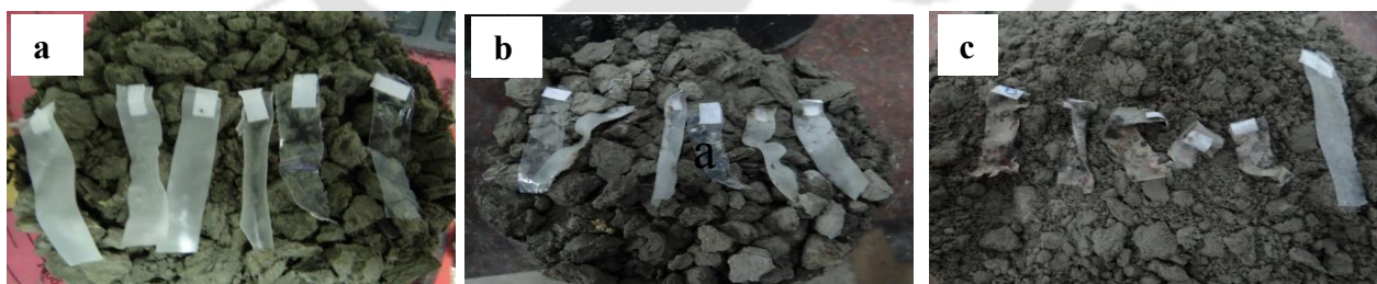
Figure 8.13. Images of soil biodegradability of starch-chitosan-nanoclay bionanocomposite films with different ratios of GFSE and LDPE for (a) 0 day, (b) 30 and (c) 60 days.
