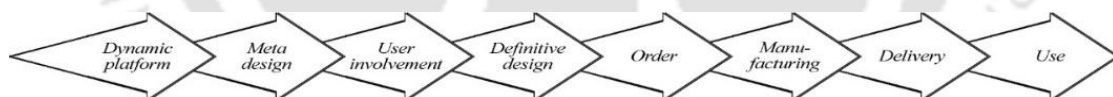
Figure 4.3.1A - A simplification of a fully 3D printable "Industrial Personalized Design and Manufacturing System" process.
