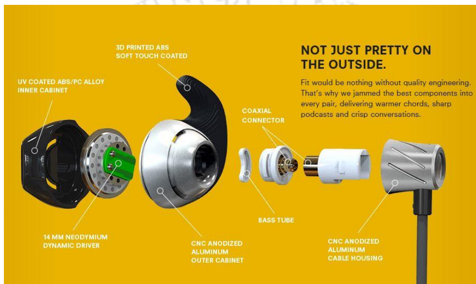
Figure 2.3X – Exploded view of Normal's earphones.
