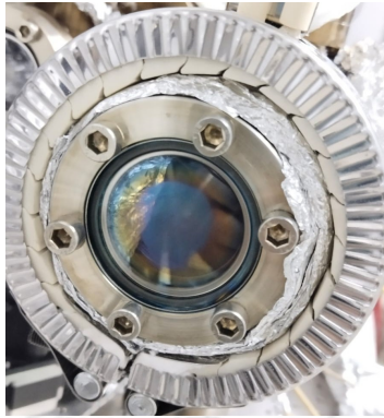
Figure 3.9: Deposition of Yb atoms on the 2D cooling stage viewports during baking. A ceramic band heater was used in an attempt to remove the coating by heating, but it was not effective.
