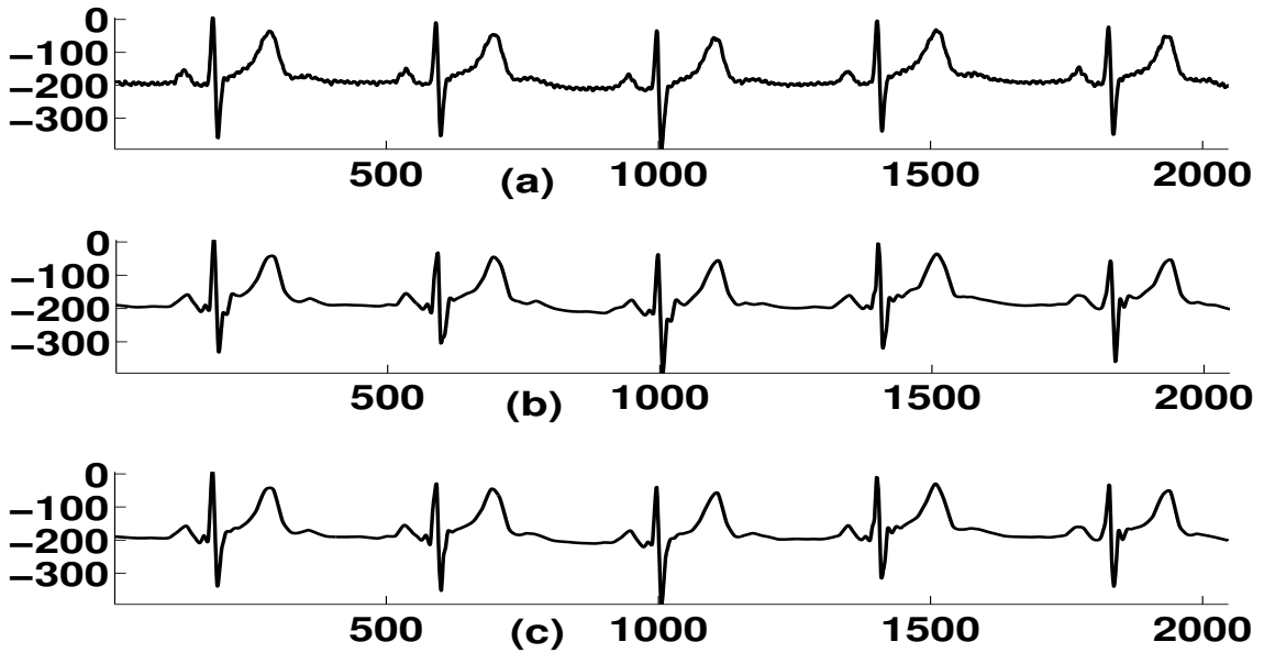
Figure 3.7: Performance of the joint thresholding and quantization strategy. (a) Original ECG signal is taken from lead II of mita record 117. (b) Reconstructed signal at threshold T_2 and T_3 selected at EPE_{F2} = 99\% and EPE_{F3} = 86\% for 7-bit quantizer. (c) Reconstructed signal at threshold T_2 and T_3 selected at EPE_{F2} = 99.9\% and EPE_{F3} = 93\% for 6-bit quantizer.
