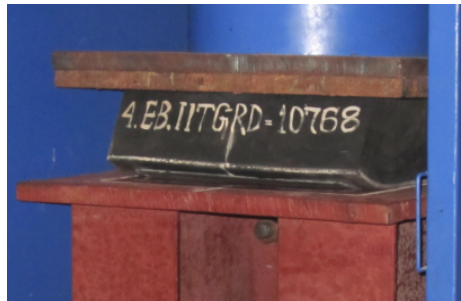
Fig. 3.4 Experimentally observed deformed shape of a typical U-FREI at applied horizontal displacement of 80 mm
