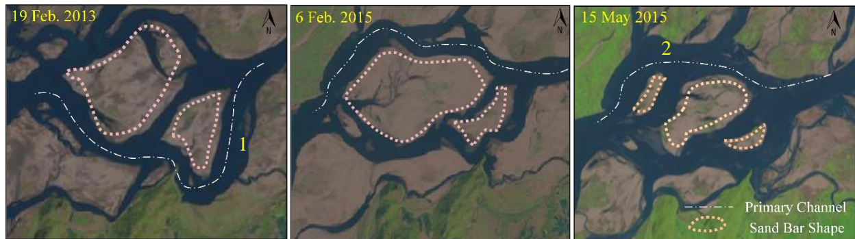
Figure 6.2 Morphological changes at Ganeshpahar from 2013 to 2015; (a) 1 is main channel in 2013; (b) 2 is main channel in 2015
