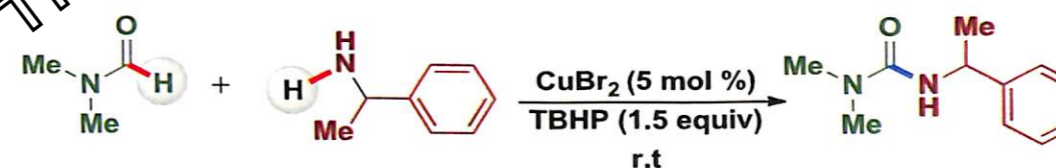
Scheme I.5.2.2.1. Cu-catalyzed coupling of C_{sp^2} -H of amide and N_{sp^3} -H of amine
