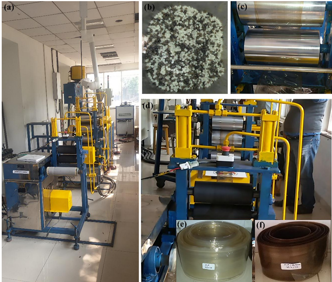
Figure 2.7. Pilot plant scale production of PLA/CH-g-OLLA bionanocomposite films;
