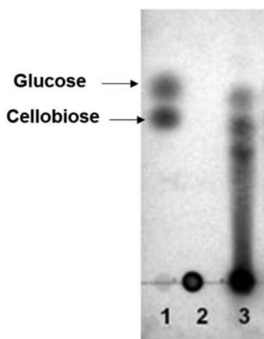
Figure 7. TLC analysis of hydrolyzed products of raw SCT and SCT cellulose by recombinant endoglucanase ( CtCel8A ), cellobiohydrolase ( CtCBH5A ) and \beta -glucosidase ( HtBgl ) enzyme from Clostridium thermocellum at 50 °C for 24 h. Lane 1, Standards (Glucose and Cellobiose), Lane 2, Unhydrolysed product of raw SCT, Lane 3, Hydrolyzed products of separated SCT cellulose.
