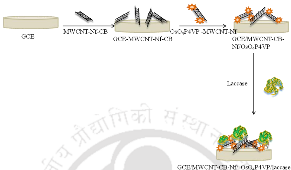
Scheme 4.1 Fabrication scheme of GCE/MWCNT-CB-Nf/OsO 4 P4VP/laccase bioelectrode.
