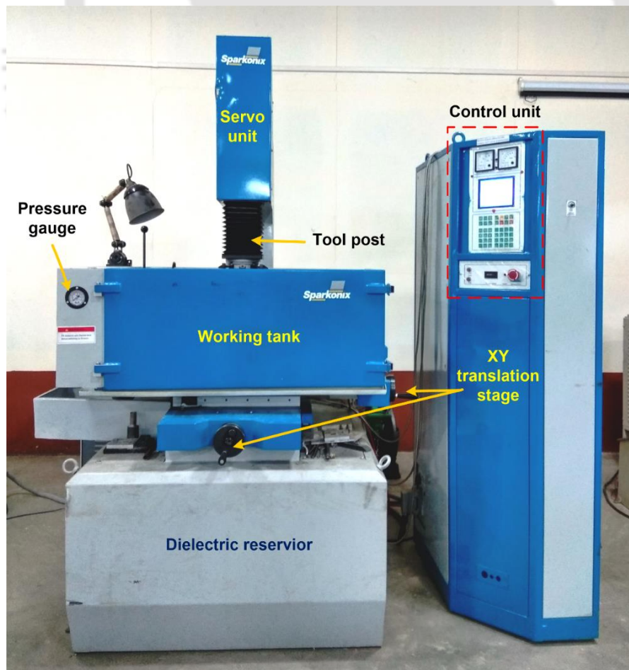
Figure 3.2 Die sinking electric discharge machine used for EDA
