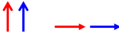
Figure 2.07. Schematic drawing of broadside and head-to-tail configurations for a pair of ferromagnetically coupled magnetic moments.
