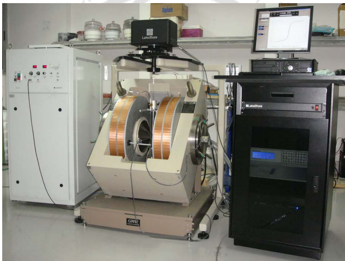
Figure 3.09. Photographic view of a vibrating sample magnetometer (Lakeshore Model 7410, USA).
