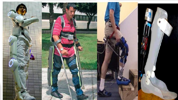
Figure 1-14. Self-Ported devices: orthoses a) HAL-5 exoskeleton, b) ReWalkTM, c) RoboKnee, d) MIT active ankle-foot orthoses (left to right)
