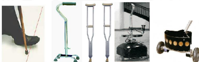
Figure 1-15. External Devices: a) Standard Canes, b) Multi-foot Cane, c) Crutches, d) Smart Cane, e) Guide Cane (left to right)
