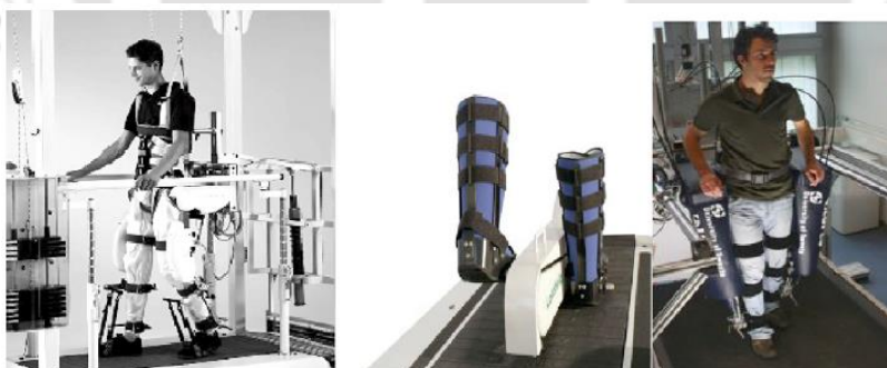
Figure 1-10. Robotic Mobility training Devices: a) Lokomat, b) LokoHelp, c) Lopes (left to right)
