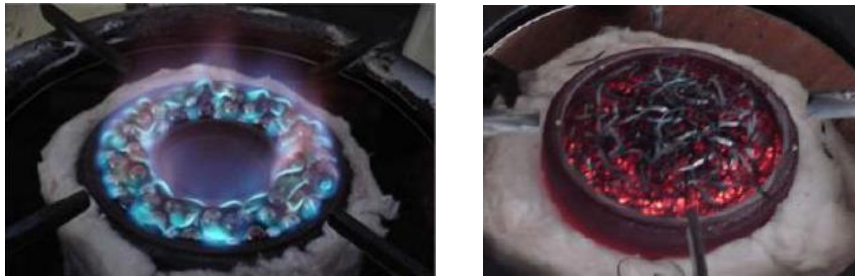
(a) Porous burners with metal balls and metal chips developed by Pantangi et al. (2007)
