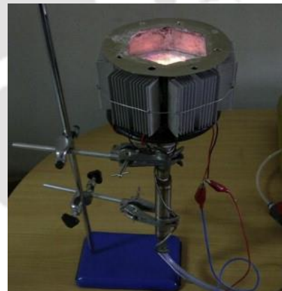
(g) PMB embedded with thermoelectric cells developed by Ismail et al. (2013)
