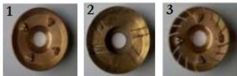
(g) 1.) Regular-shaped burner, 2.) Cyclone 1-shaped burner, 3.) Cyclone 2-shaped burner (Syamsuri et al., 2015)
