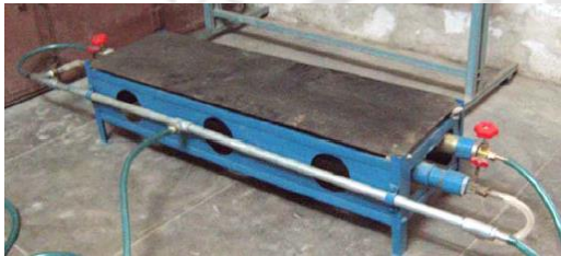
(e) Biogas stove for baking developed by Kurchania et al. (2010)
