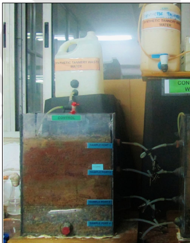
Figure 3.10: Photograph of the experimental setup showing VSSF CWs operated under continuous mode: (a) Planted unit (b) Control unit
