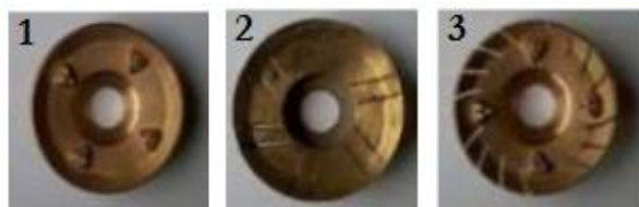
g) 1.) Regular-shaped burner, 2.) Cyclone 1-shaped burner, 3.) Cyclone 2-shaped burner (Syamsuri et al., 2015)
