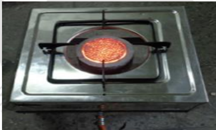
Fig. 2.2 Domestic Porous Radiant Burner developed by Mishra and Muthukumar (2018)
