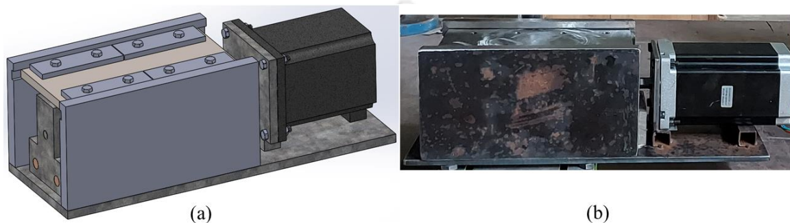
Fig. 3.15 Depicts the (a) CAD model and (b) final assembled welding bed
