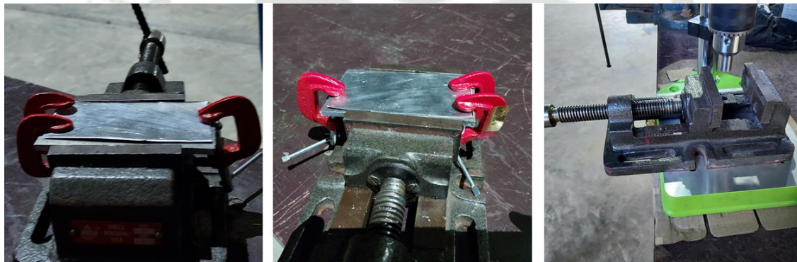
Fig. 3.19 Portable bench vice and 1-inch C-type clamping arrangement
