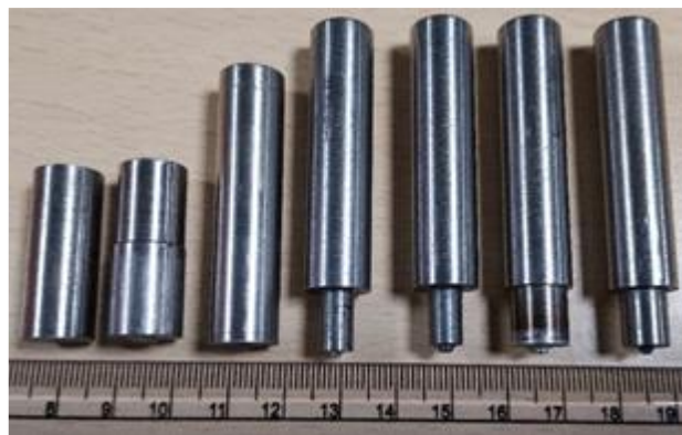
Fig. 3.3 Representation of various tools used for FSW with varying shoulder and pin geometry
