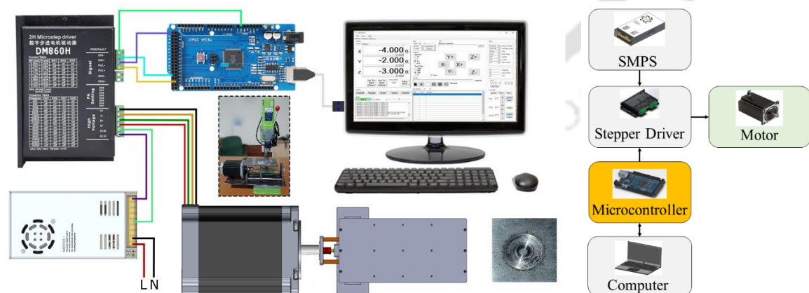
Fig. 3.21 Circuit diagram to control the welding bed movement.
