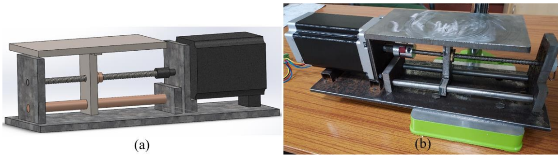
Fig 3.14 Depicts the (a) CAD model, and (b) photograph of initial welding bed assembly
