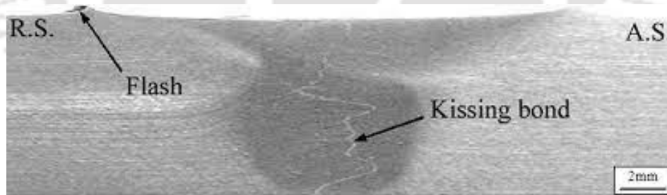
Fig. 2.5 Cross-sectional representation of kissing bond defect during AA5083 FSW (Zhou, Yang and Luan, 2006)
