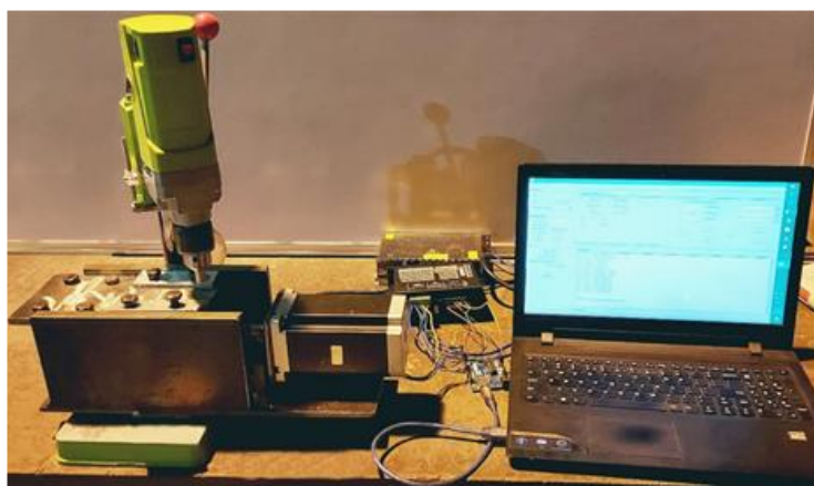
Fig. 3.5 Complete experimental setup developed for the \mu -FSW
