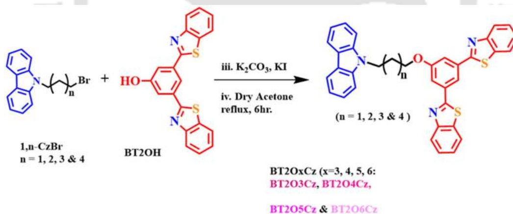
Scheme 4.3. 2,2'-(5-(3-(9H-carbazol-9-yl)alkoxy)-1,3phenylene)bis(benzothiazole) [BT 2 OxCz, x=3,4,5,6].
