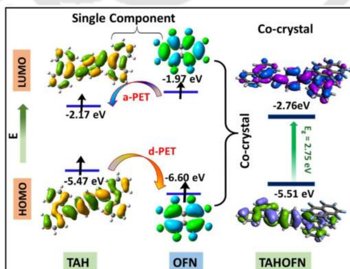
Figure A3.3. Mechanism of weak fluorescence (a-PET & d-PET) for TAHOFN by DFT/TD-DFT calculated HOMO/LUMO energy band diagram for conformer TAH and OFN.
