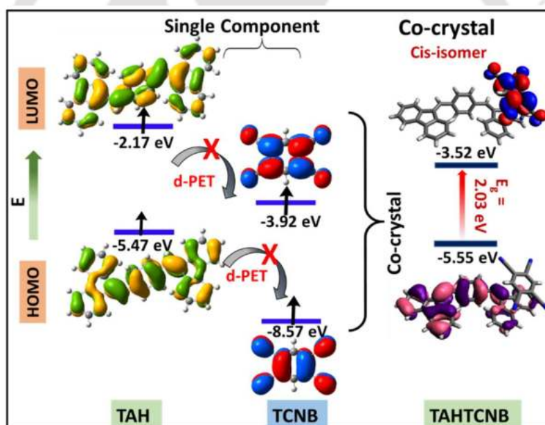
Figure A3.5. Red fluorescence and strong narrow band CT mechanism for the cis-isomeric co-crystals of TAHTCNB by DFT/TD-DFT calculated HOMO/LUMO energy band diagram for the conformer TAH and TCNB.
