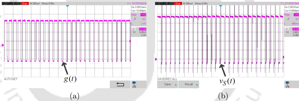
Figure 3.15: (a) Gate signal ( g(t) ) of DC/MF converter. (b) Switched output voltage of DC/MF converter.
