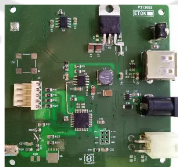
Figure 3.17b Smart battery (Li-ion) PCB Prototype
