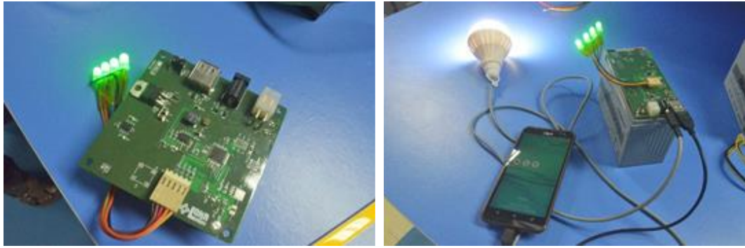
Fig 3.28 a. Lithium-ion and b. VRLA smart battery modules
