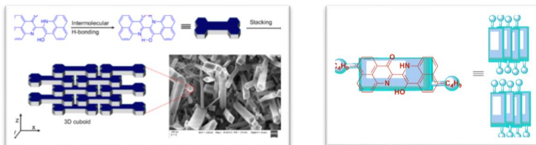
Fig 3. 3 Difference in the aggregation mechanism of PNI and butylPNI
