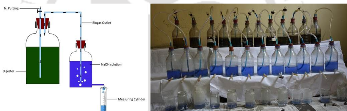
Fig. 3.2. Experimental diagram of anaerobic BMP setup
