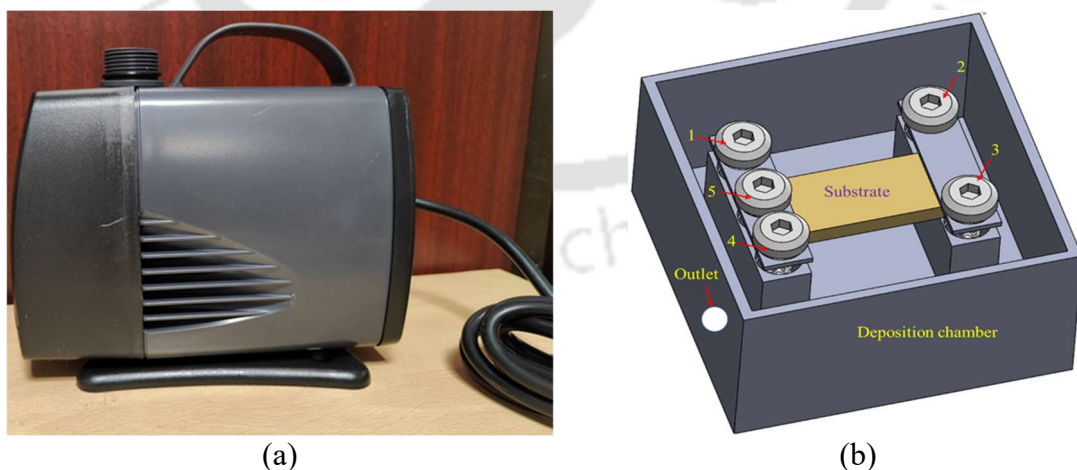
Fig. 3.5 (a) Submersible pump and (b) deposition chamber of SJED setup
