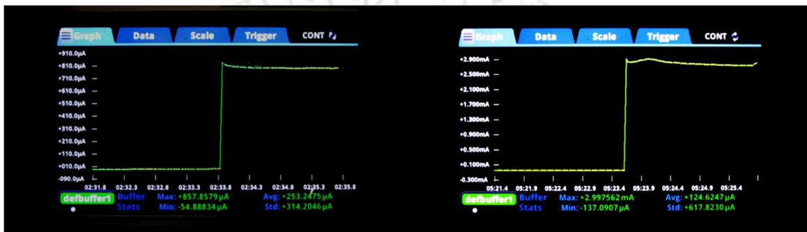
(a) (b) Fig. 3.3 Wave images captured by DMM at (a) 3V and (b) 5V
