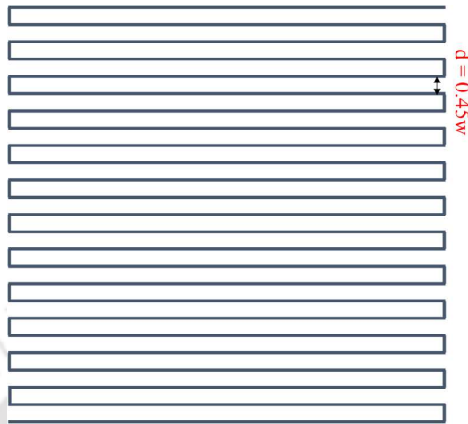
Fig. 5.9 Raster tool path for coating by SJED technique
