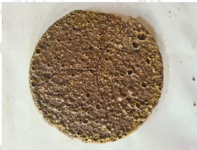
Fig. 4.6 Picture showing abnormal cysts like lesions developed over the surface of membrane.
