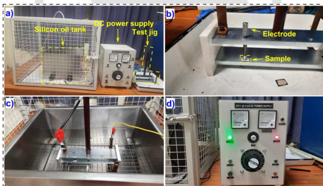
Fig. 4.9: a) Electrode poling setup, b) sample under loading condition, c) electrical connections before poling, d) ongoing poling operation.
