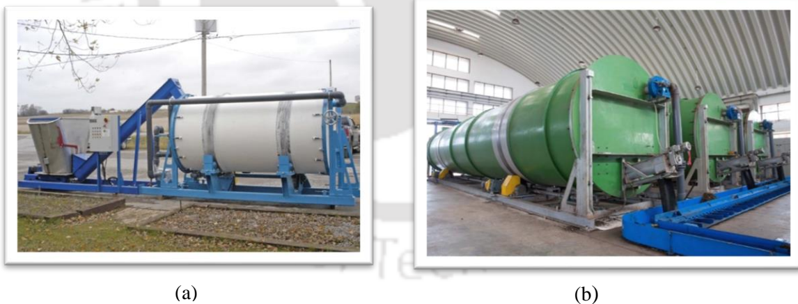
Fig. 2.16. In-vessel composter design (a) Small scale in vessel composter ( https://xactsystemscomposting.com/images/ ) & (b) Pilot scale in-vessel composter ( https://sfcenvironment.com/orex )
