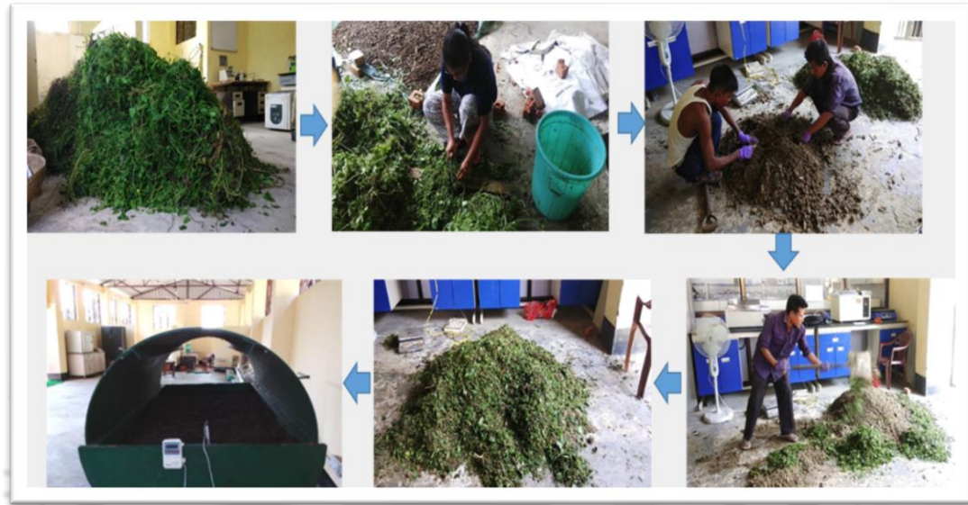
Fig. 4.4 Preparation of the feeding mixture for the rotary drum composter
