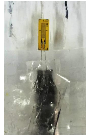
Figure 6.4 A typical 2 mm gage length, pre-wired strain gage
