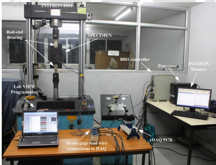
Figure 6.14 Photograph of complete experimental set-up
