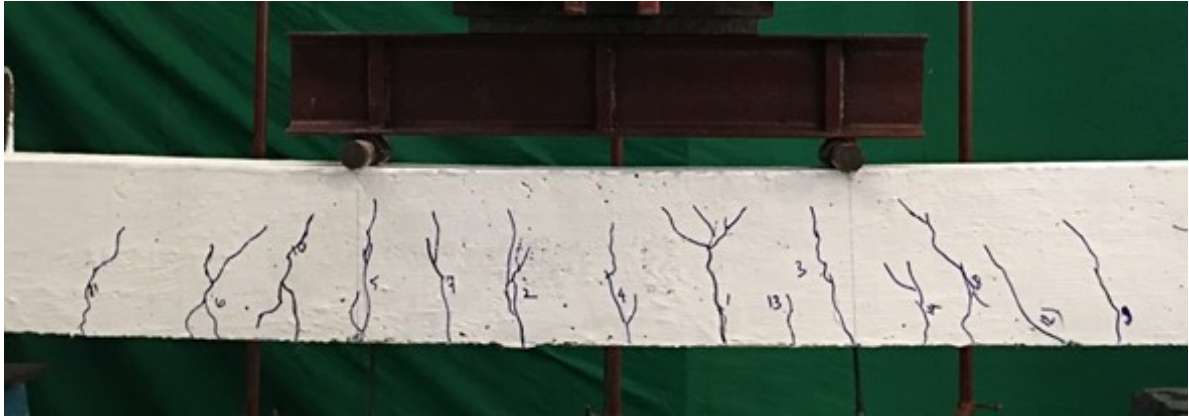
Figure 6.12 (a): Cracks in fully damaged RC beam, B10.
