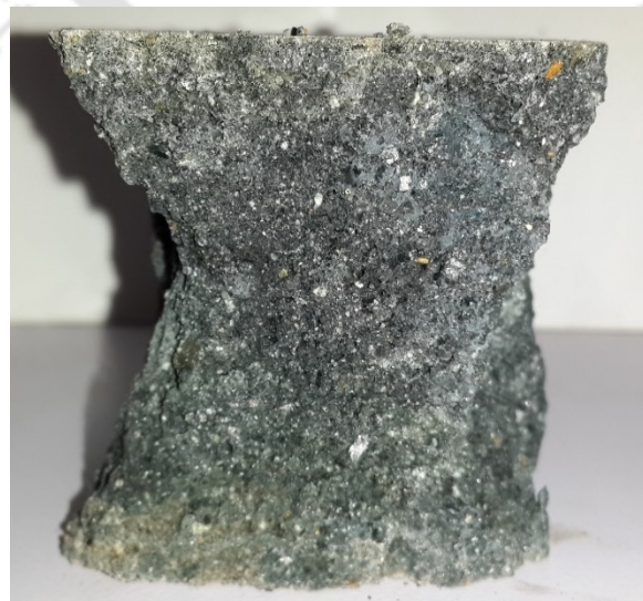
Figure 3.27 (d): Crushed mortar cube at 28 days (GM12).
