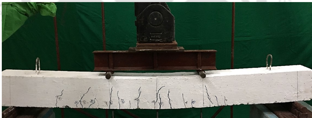
Figure 5.17 (b): Cracks in GPM repaired beam, B2R
