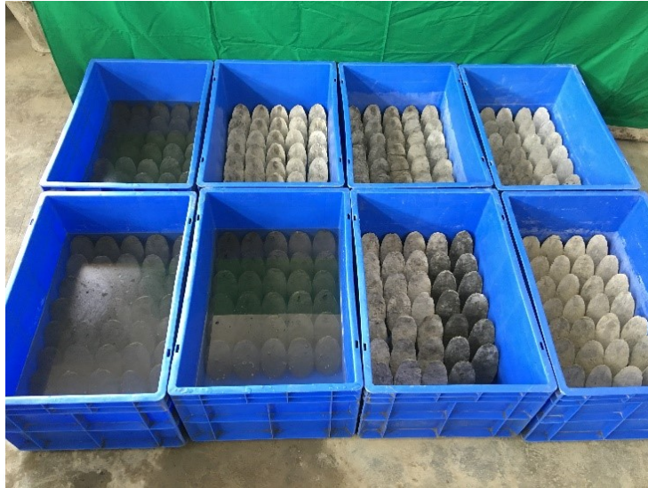
Figure 4.7: Curing of PCC substrates in water and open air.
