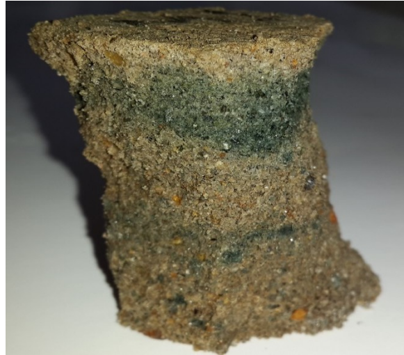
Figure 3.27 (b): Crushed mortar cube at 3 days (GM12).
