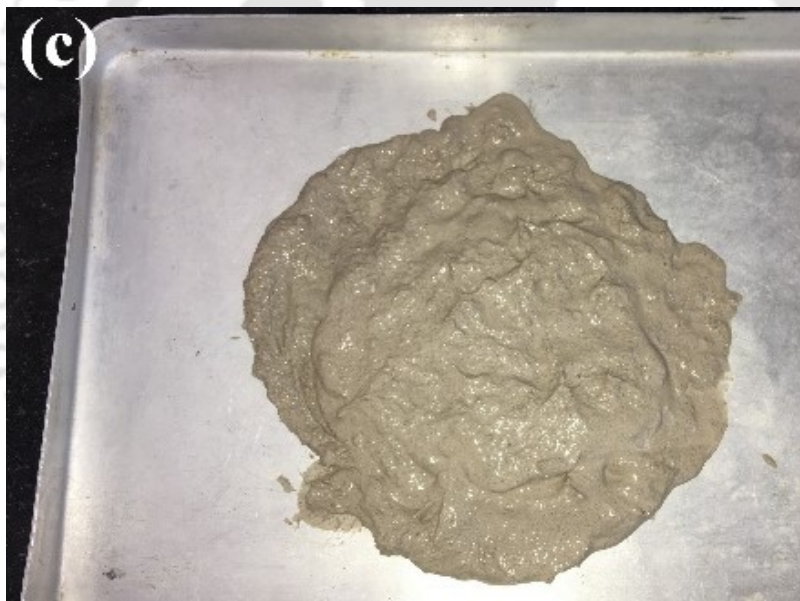
Figure 3.16 (c): Appearance of fresh geopolymer mortar, GM 21 which consisted of 3.0 % SN based SP.
