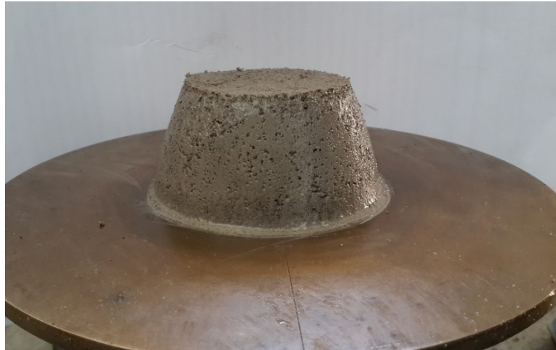
Figure 3.9 (a): Flow table test (Before the jolting of the flow table).
