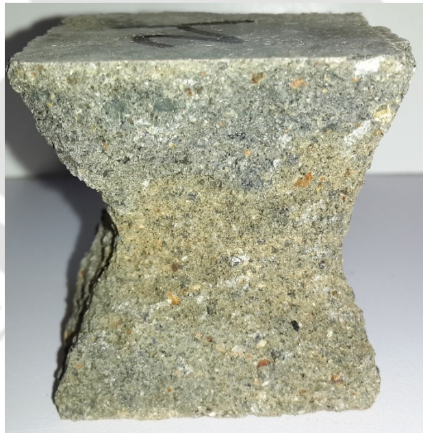
Figure 3.27 (a): Crushed mortar cube at 3 days (GM11).
