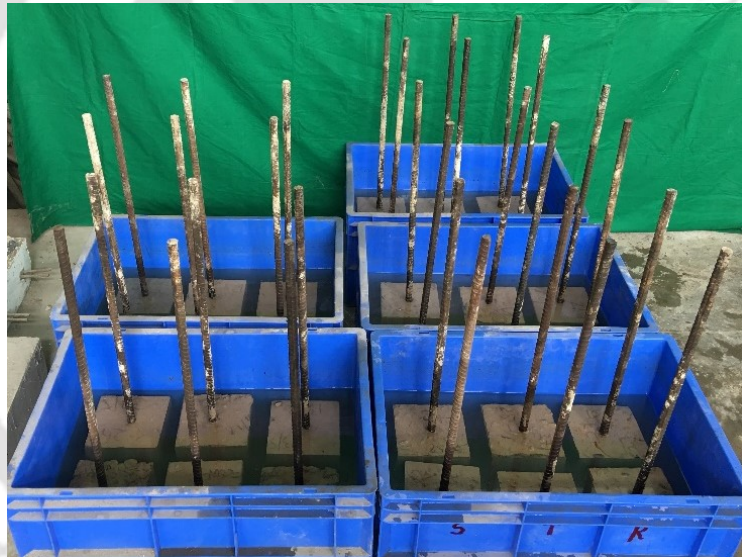
Figure 4.5: Pull-out test specimens under curing.
