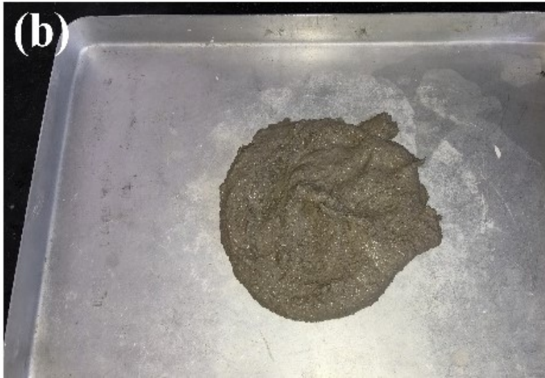
Figure 3.16 (b): Appearance of fresh geopolymer mortar, GM 19 which consisted of 1.5 % SN based SP.
