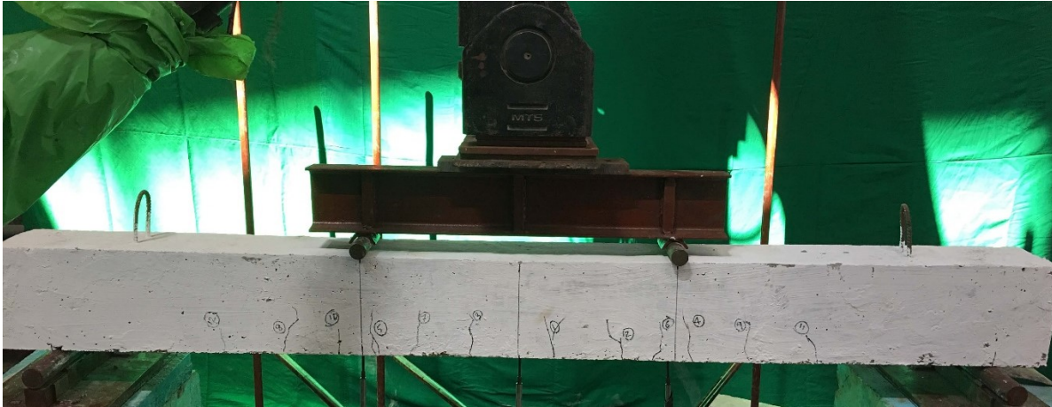
Figure 5.7: Cracks in partially damaged RC beam.
