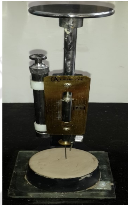
Figure 3.7: Vicat apparatus used for setting time test.
