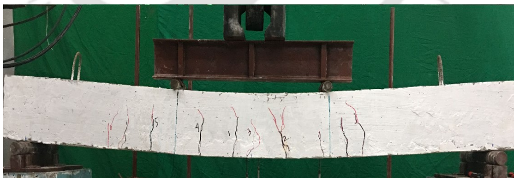
Figure 5.22 (b): Cracks in GPM repaired beam, B7R.
