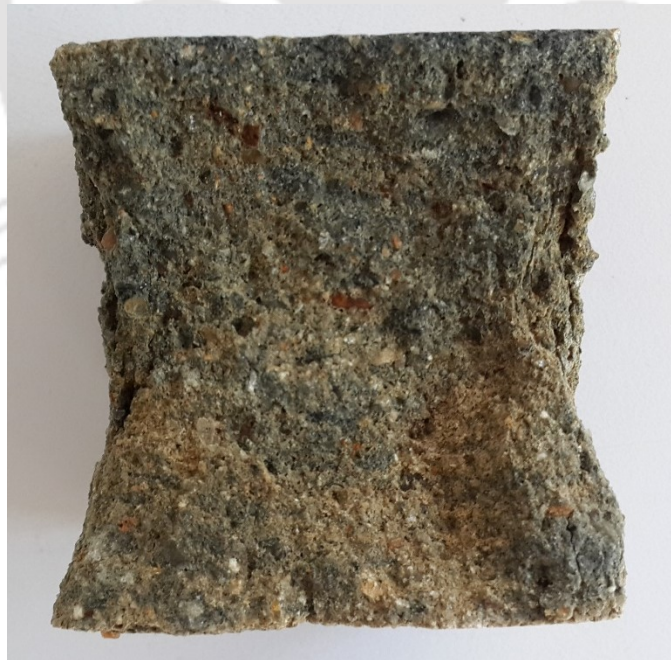
Figure 3.24 (a): Crushed mortar cube at 3 days (GM5).
