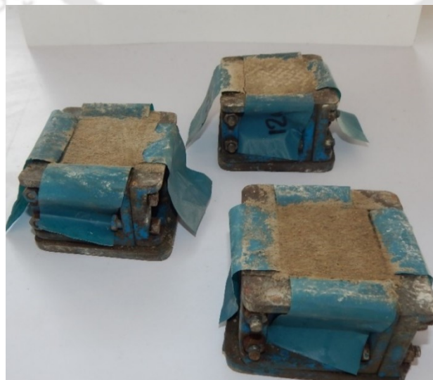
Figure 3.4: Geopolymer mortar inside the cube mould.
