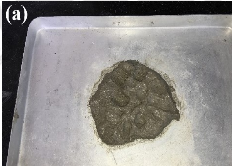
Figure 3.16 (a): Appearance of fresh geopolymer mortar, GM 17 which consisted of 0.5 % SN based SP.
