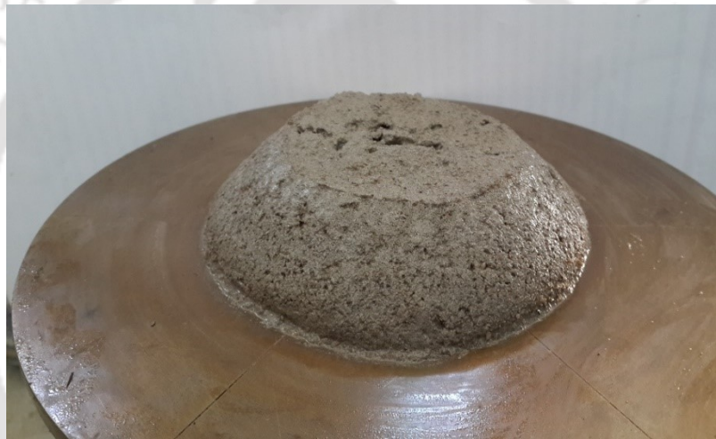
Figure 3.9 (b): Flow table test (After the jolting of the flow table).
