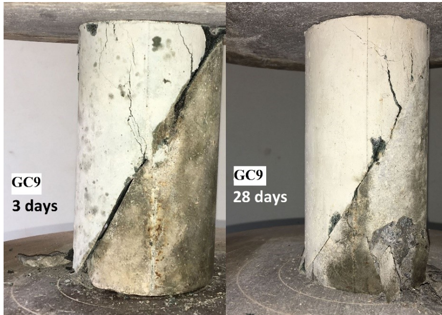
Figure 4.29: Slant shear test specimens with cracks in GPC and PCC region.
