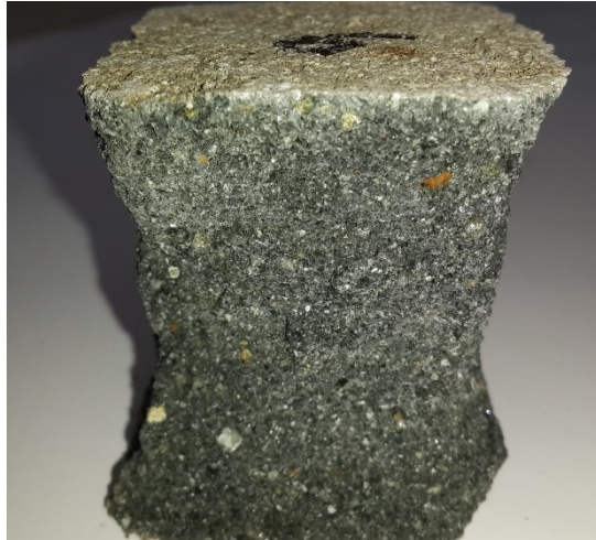
Figure 3.24 (e): Crushed mortar cube at 3 days (GM6).
