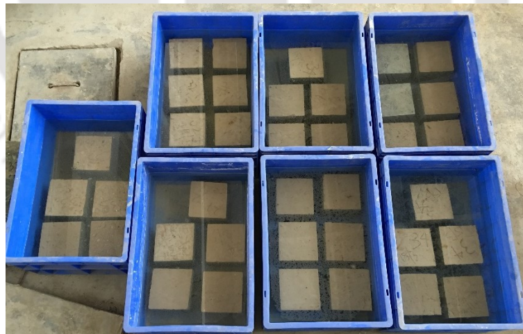
Figure 4.2: Concrete cubes under curing.
