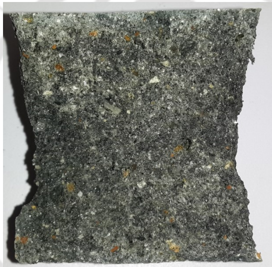
Figure 3.24 (f): Crushed mortar cube at 3 days (GM8).
