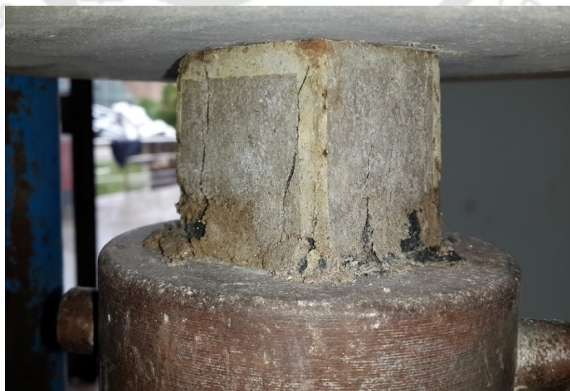
Figure 3.10: Geopolymer mortar cube crushed in the compressive testing machine.
