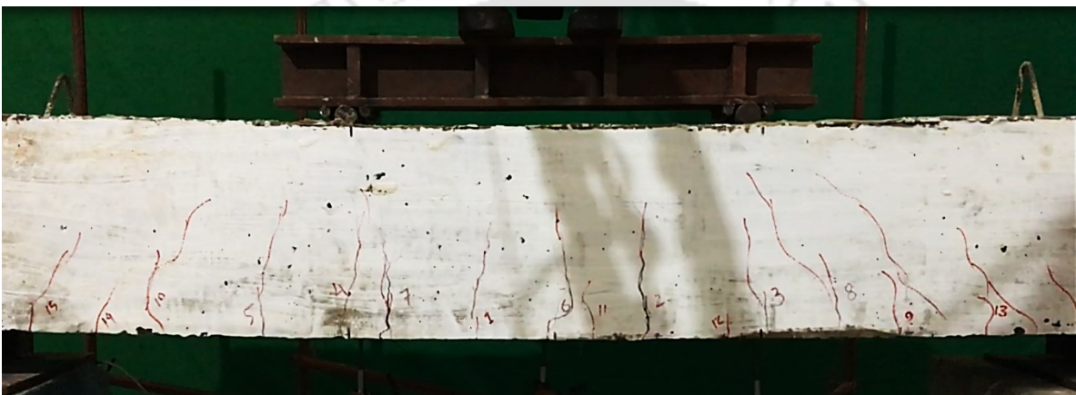
Figure 6.15 (b): Cracks in GPC jacketed RC beam, B13J.
