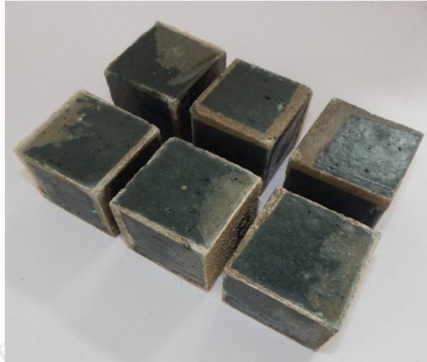
Figure 3.5: Geopolymer mortar cubes ready for curing after 24 hours from casting time.
