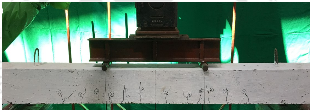
Figure 5.22 (a): Cracks in controlled beam, B7.
