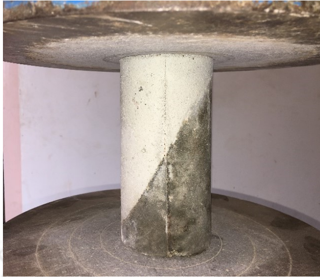
Figure 4.10: Test setup for slant shear test.
