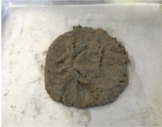
Figure 3.3: Geopolymer mortar in fresh state.
