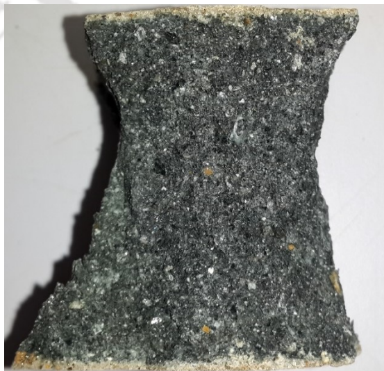
Figure 3.24 (g): Crushed mortar cube at 28 days (GM6).
