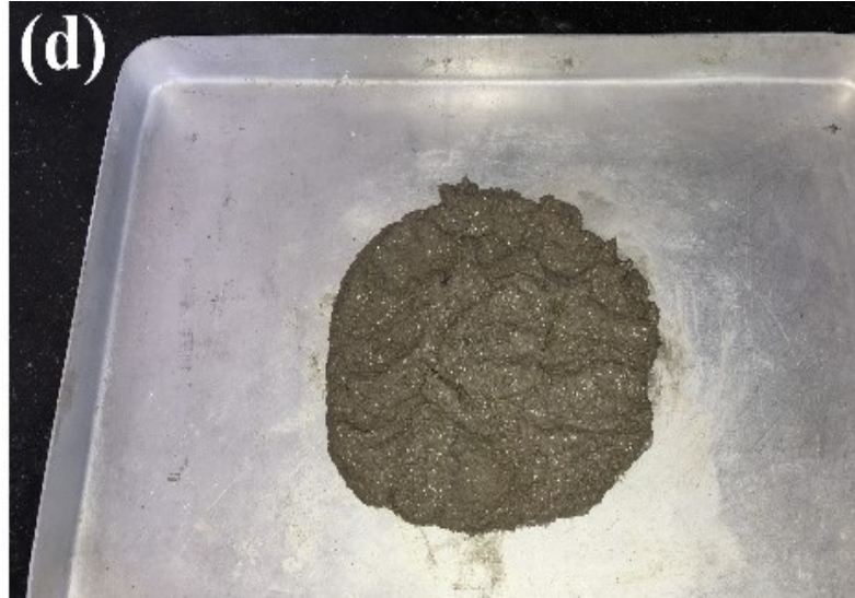
Figure 3.16 (d): Appearance of fresh geopolymer mortar, GM 22 which consisted of 3.0 % PE based SP.
