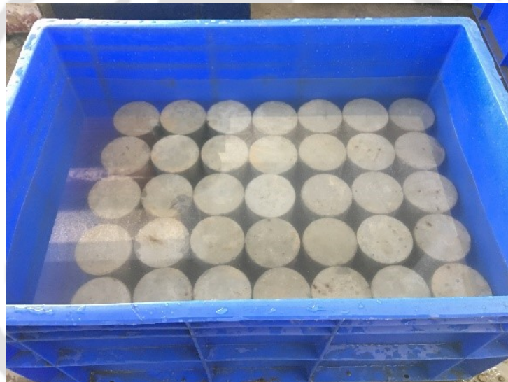
Figure 4.8: Curing of slant shear specimens in water.
