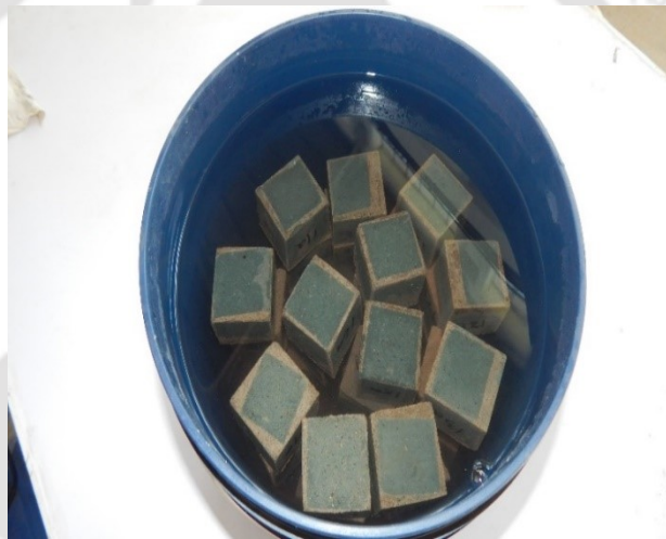
Figure 3.6: Geopolymer mortar cubes submerged inside water tank for curing.
