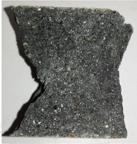
Figure 3.24 (h): Crushed mortar cube at 28 days (GM8).
