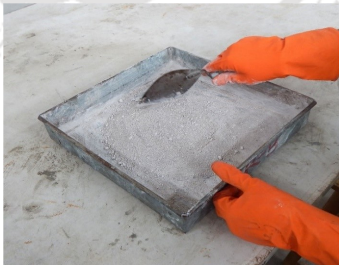
Figure 3.2: Dry mix consisting of UGGBS, FA and fine aggregate.
