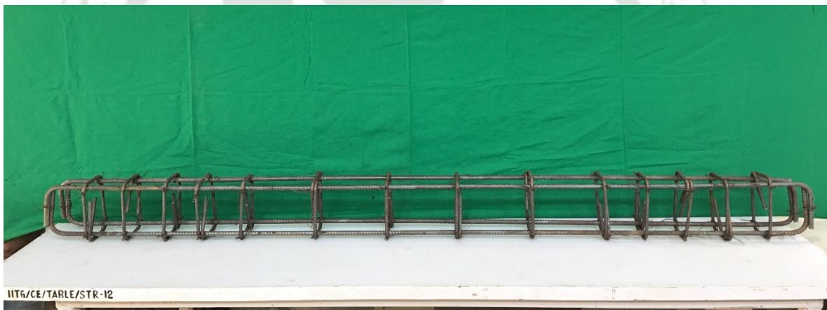
Figure 5.3: Reinforcement provided in the RC beams.
