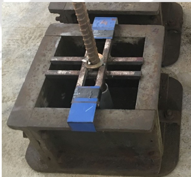
Figure 4.3: Mould for pull-out test specimens.
