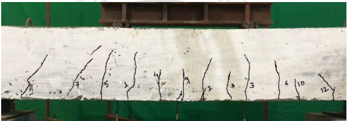
Figure 6.12 (b): Cracks in GPC jacketed RC beam, B10J.
