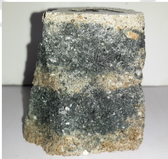
Figure 3.24 (d): Crushed mortar cube at 28 days (GM7).
