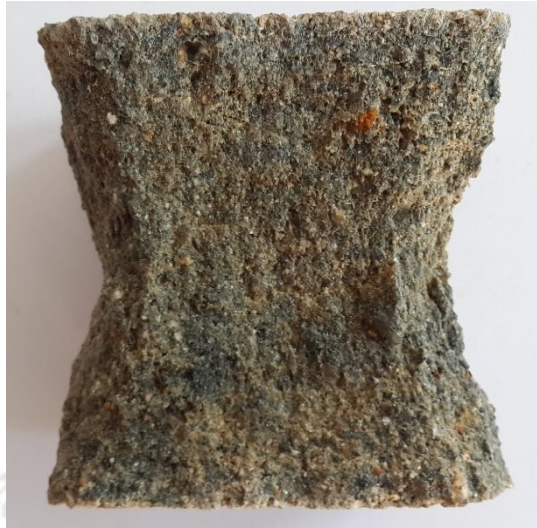
Figure 3.24 (b): Crushed mortar cube at 3 days (GM7).
