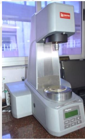
Figure 2.1 Photograph of the rheometer [manufacturer: Anton Paar (Germany), model: Physica MCR 301].
