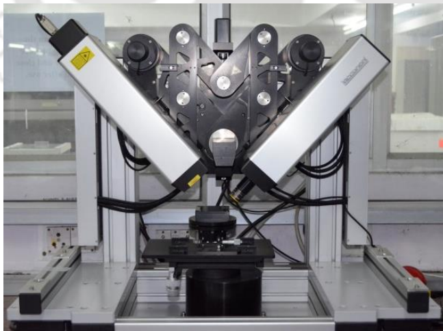
Figure 2.4 Photograph of the ellipsometer.
