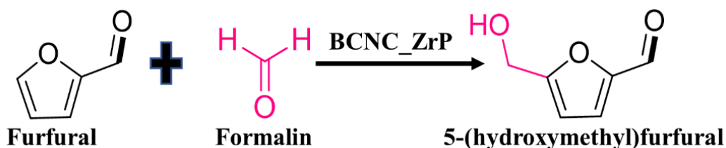
Scheme 5.1. Reaction mechanism showing hydroxymethylation of furfural to obtain HMF.
